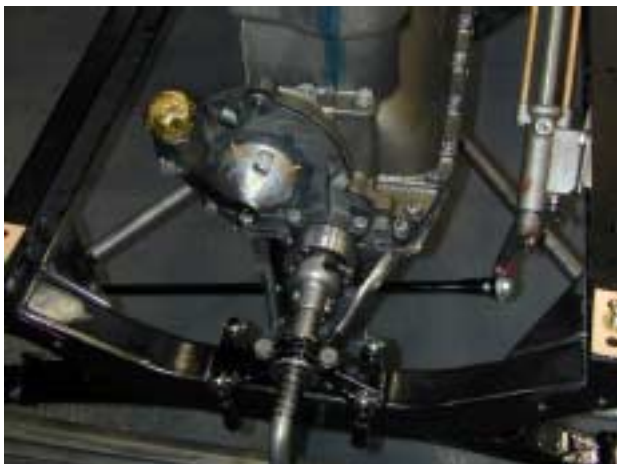
Note the counter-balanced crankshaft. These were made in New Zealand and can be had from most T parts suppliers for a bit over a grand.
