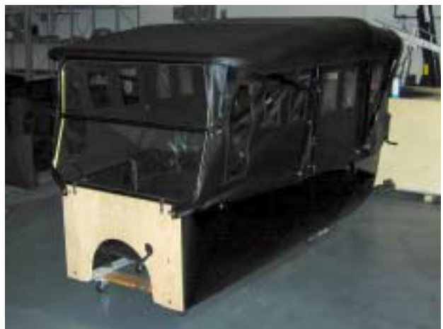
Completely upholstered and topped body waiting for a completed chassis.
