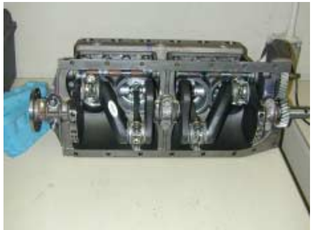
Note the counter-balanced crankshaft. These were made in New Zealand and can be had from most T parts suppliers for a bit over a grand.
