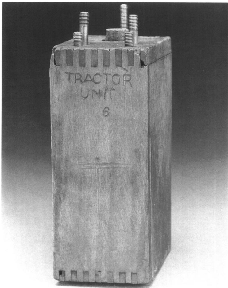
Photo 23: Special coil units for the Fordson tractor were marked "Tractor units" from 1920 to 1922. These coils differed from regular Model T production in that they used a larger condenser and the melting point of the insulating compound (Ford Hydrolene) was higher than the standard material used in Ford cars and trucks.
