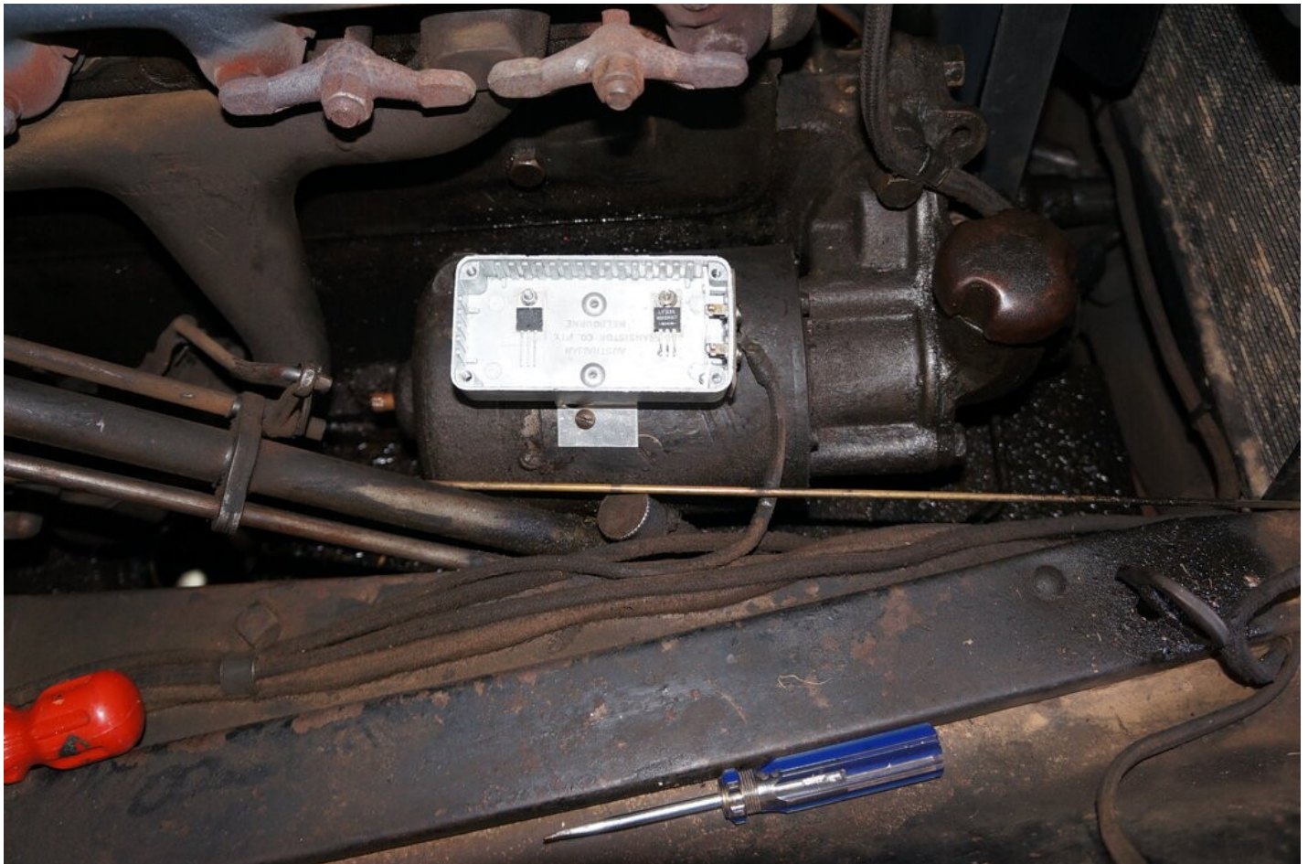
How the regulator mounts to the generator in place of the original cutout. MOSFET and cutout diode have been screwed to the box for heatsinking.
