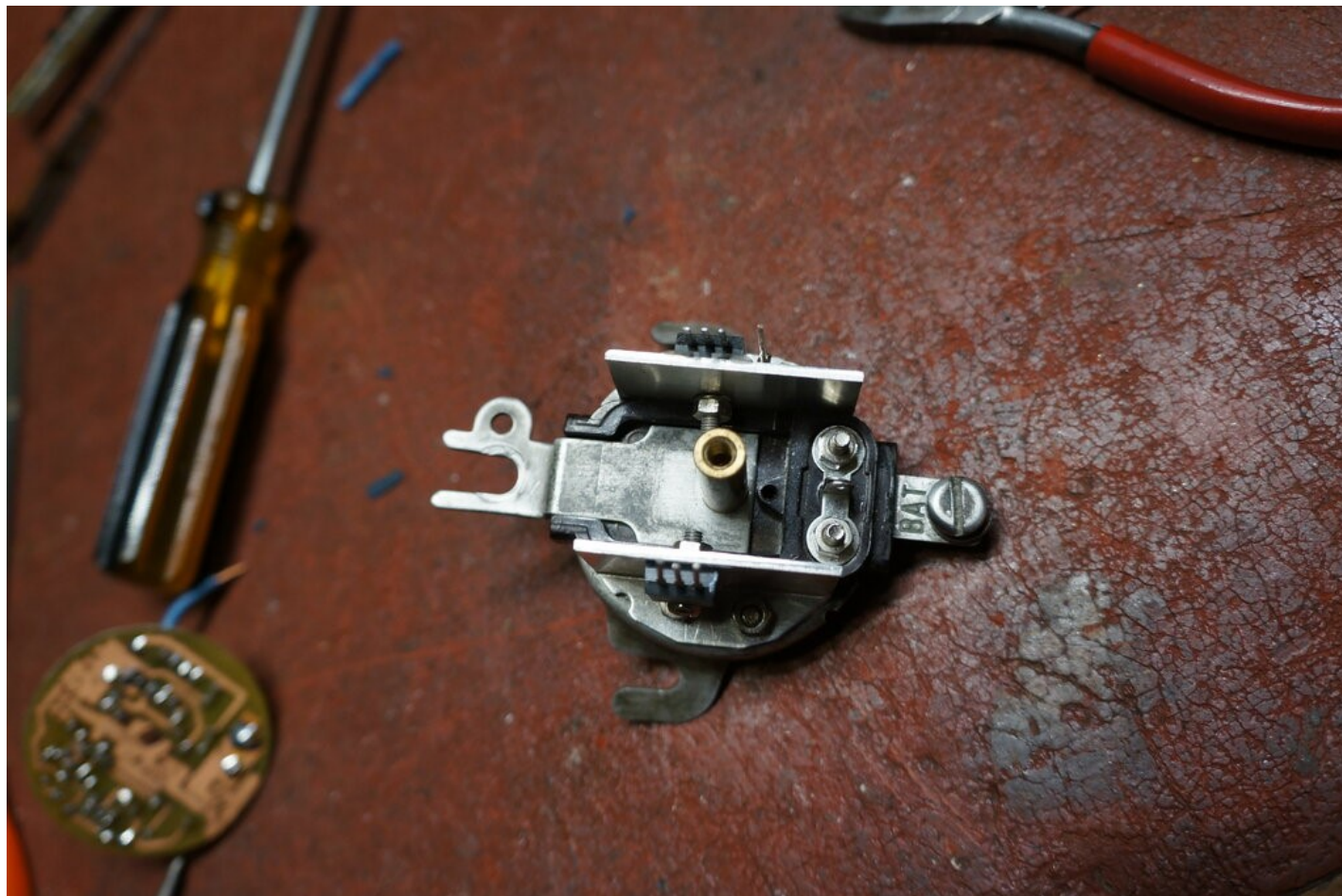
Heatsink brackets with diode and MOSFET attached. Central pillar supports PCB.
