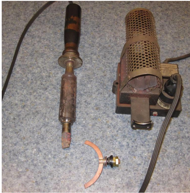
Figure 3 Typical 250-Watt Soldering Iron
