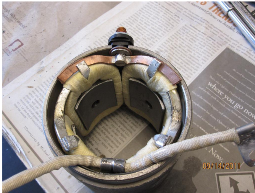
Figure 6 Terminal Bolt Properly Positioned in Case Wall Relief
