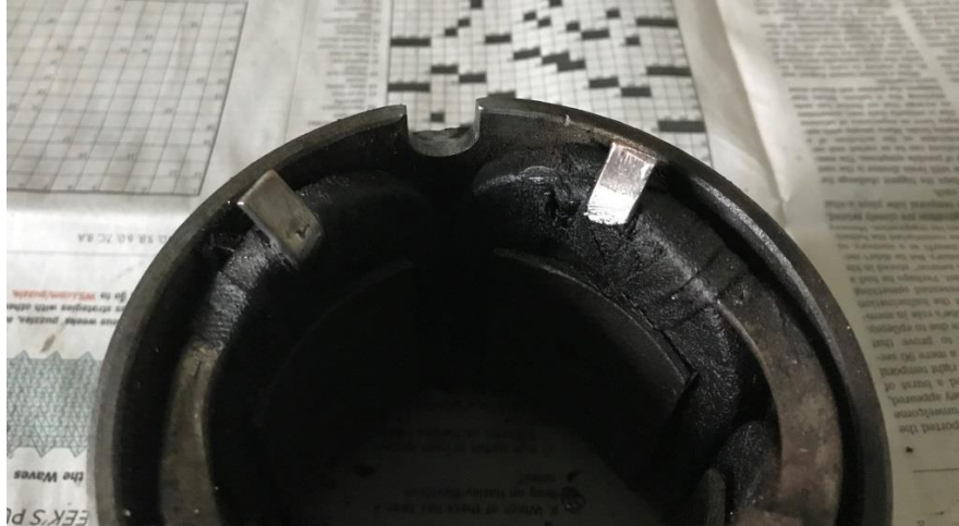
Figure 4 Starter Case Ready for New Terminal Bolt Installation
