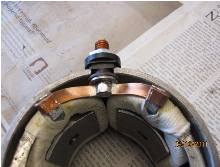
Figure 8 New Terminal Bolt Installed and Ready for Soldering
