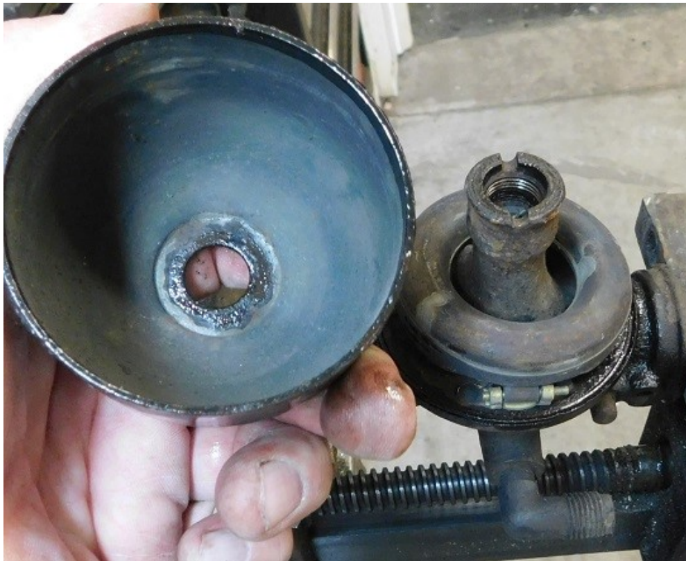
Inside the bowl is just what we like – no rust and a misadjusted float that probably caused this carburetor to be removed long ago.
