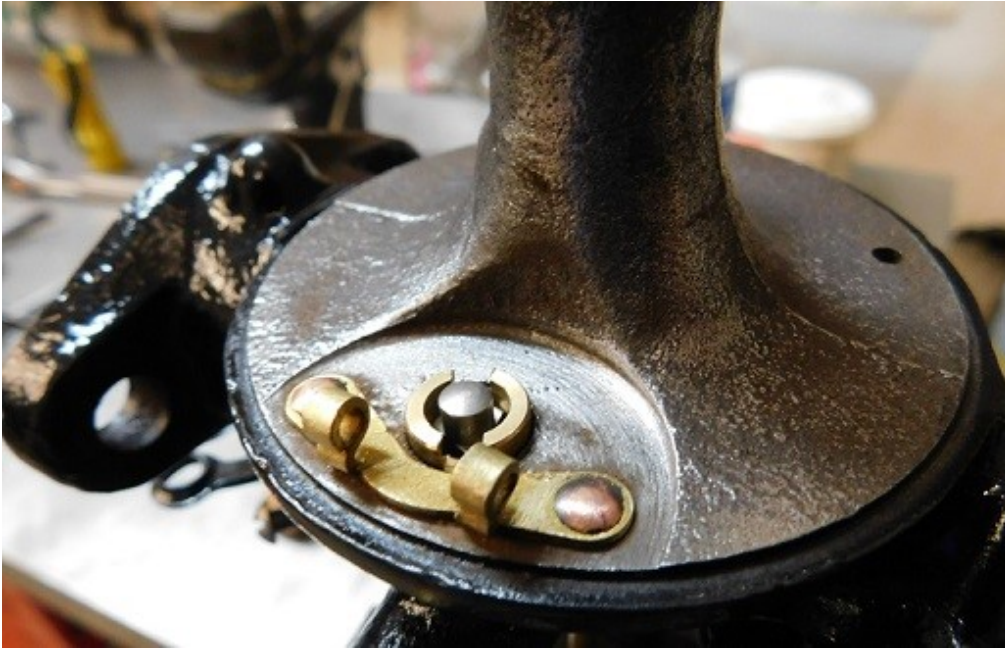
The needle should sit in the seat just about flush, barely protruding where the float touches it..
