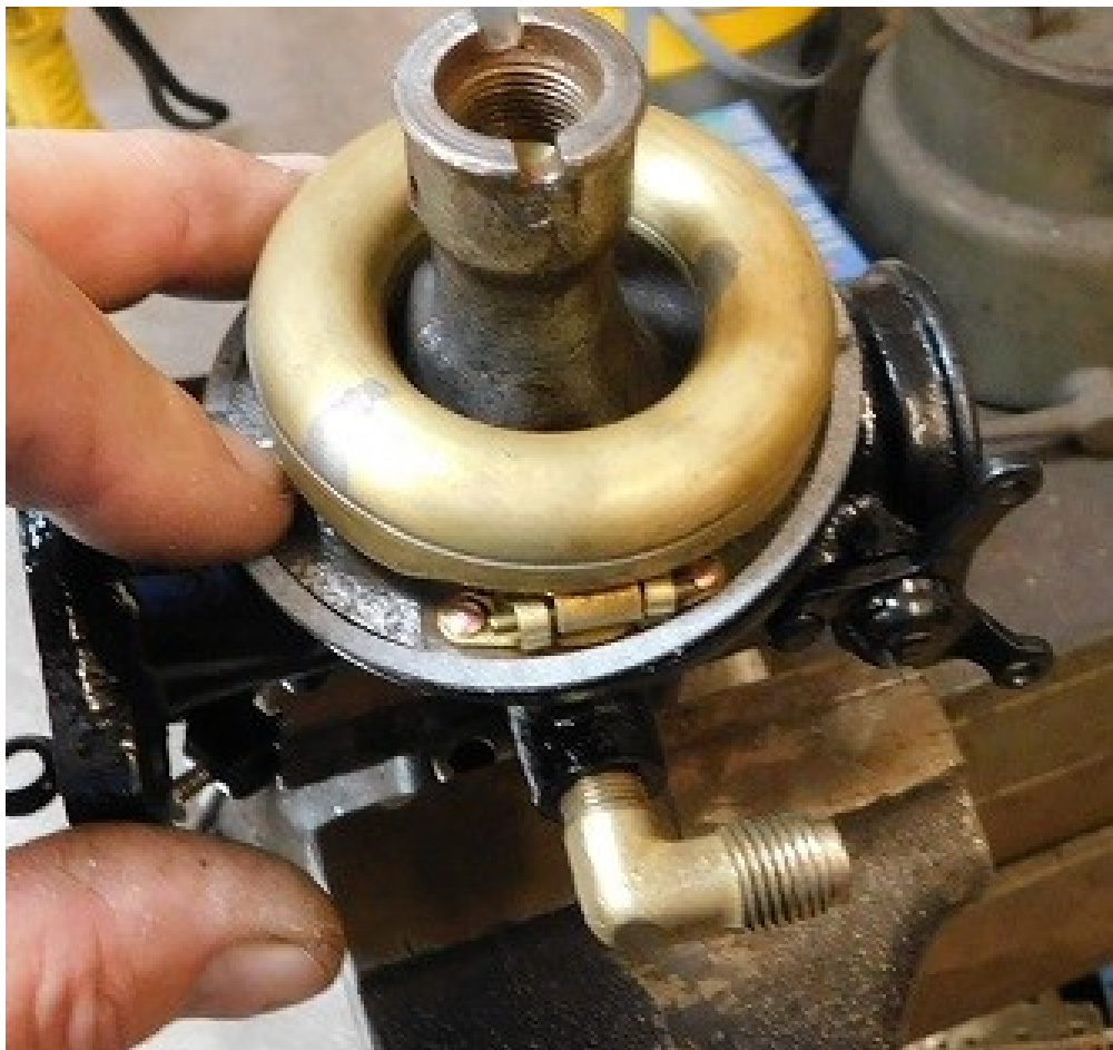
A new bowl gasket is checked for fit.
