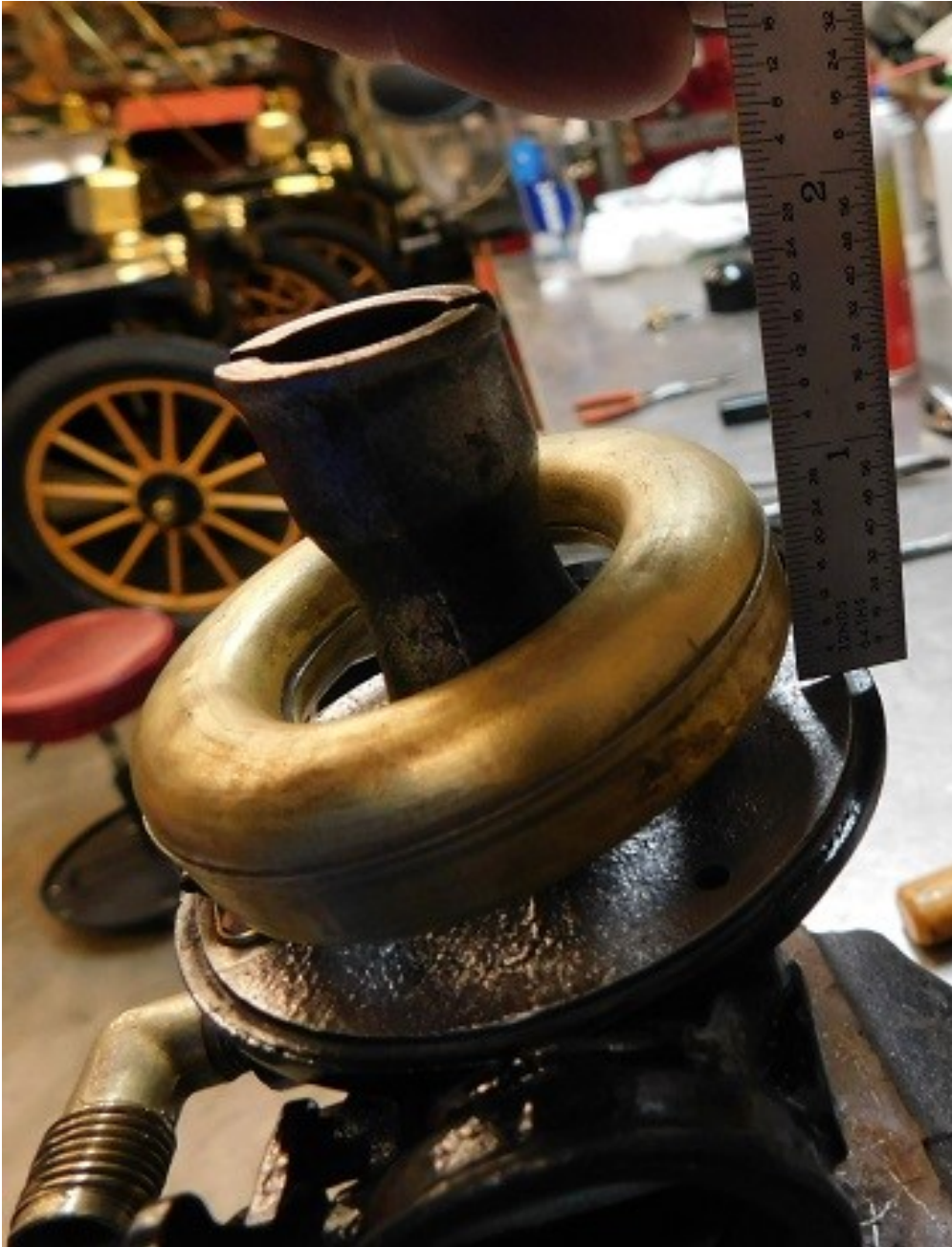
The float dimension should be 1/4" at a point 180 degrees from the inlet valve. Ours needs adjustment.
