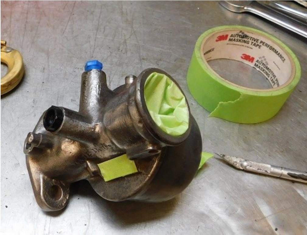
The carburetor bowl is installed temporarily using the old gasket and then we spend a little time masking it off for paint.
