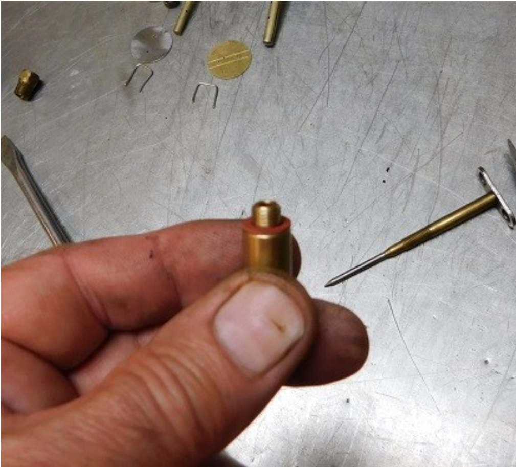
The gasket is placed on the new fuel inlet seat so that it can be installed.
