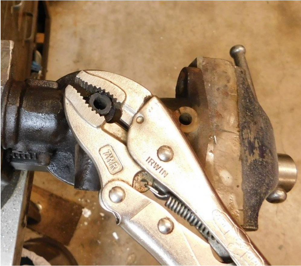
The tension adjuster for the mixture needle is stuck. We had to use Vice Grip pliers to get it out.
