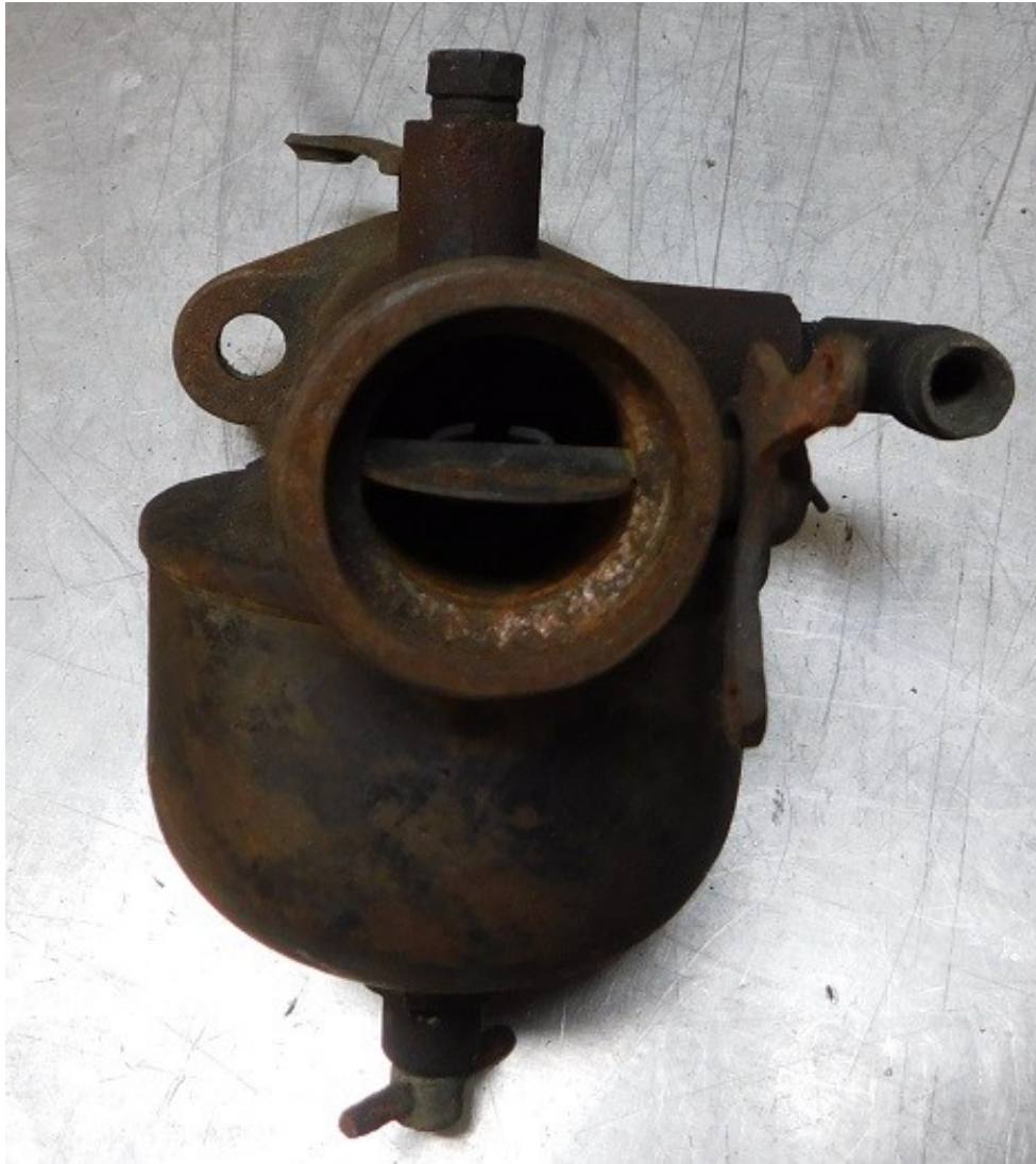
While the choke lever was present and usable, the choke return spring was broken.
