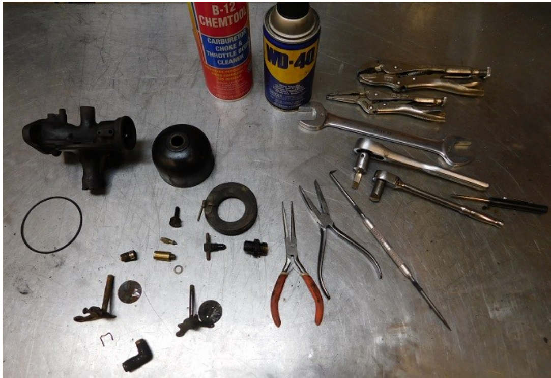
All the parts that were removed are now ready for their 24 hour stay in the carb cleaner can.
