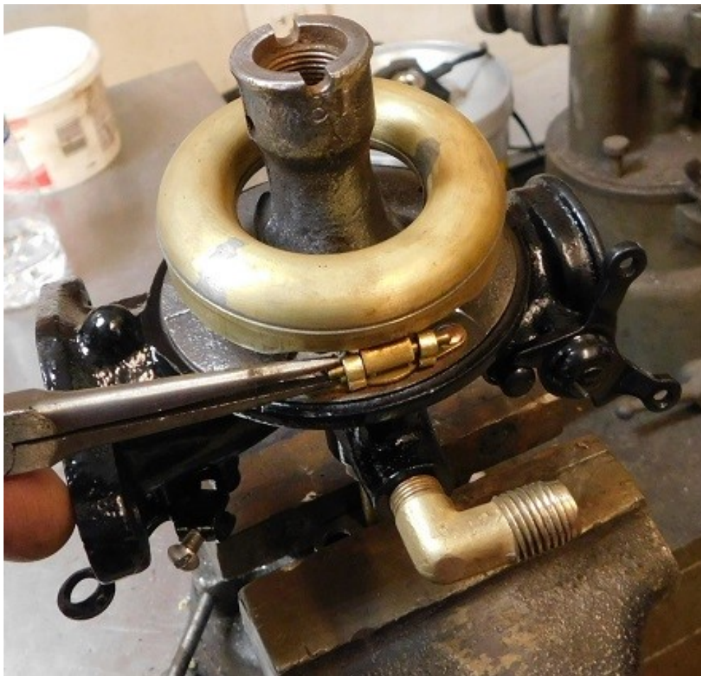
We install the float and secure it with its hinge pin.
