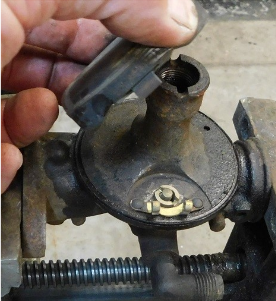
This exposes the fuel inlet needle and seat assembly.
