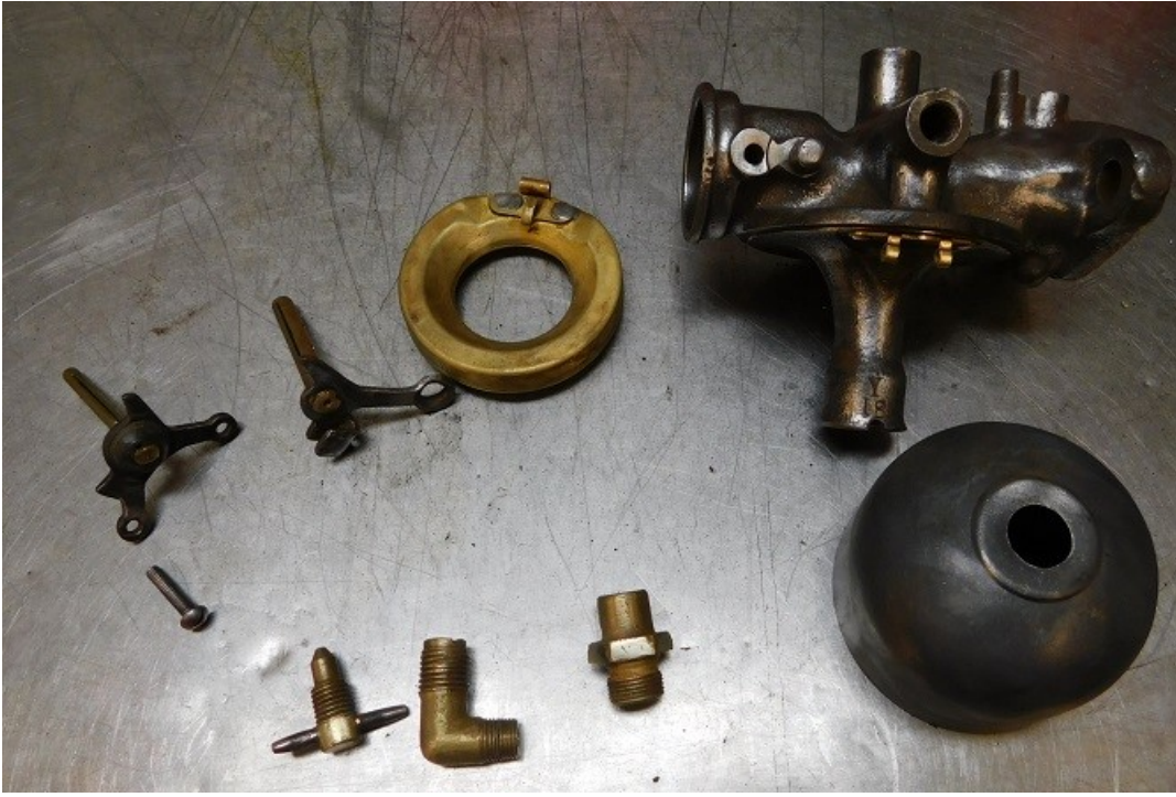
The parts are left overnight, then scrubbed with Scotch Brite and rinsed in hot water.
