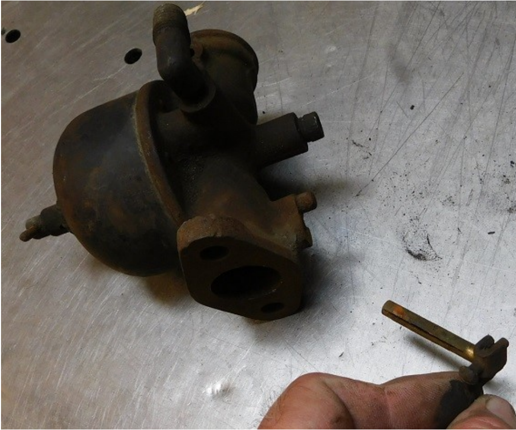
The throttle shaft then comes right out. This is a really good one with minimal wear.
