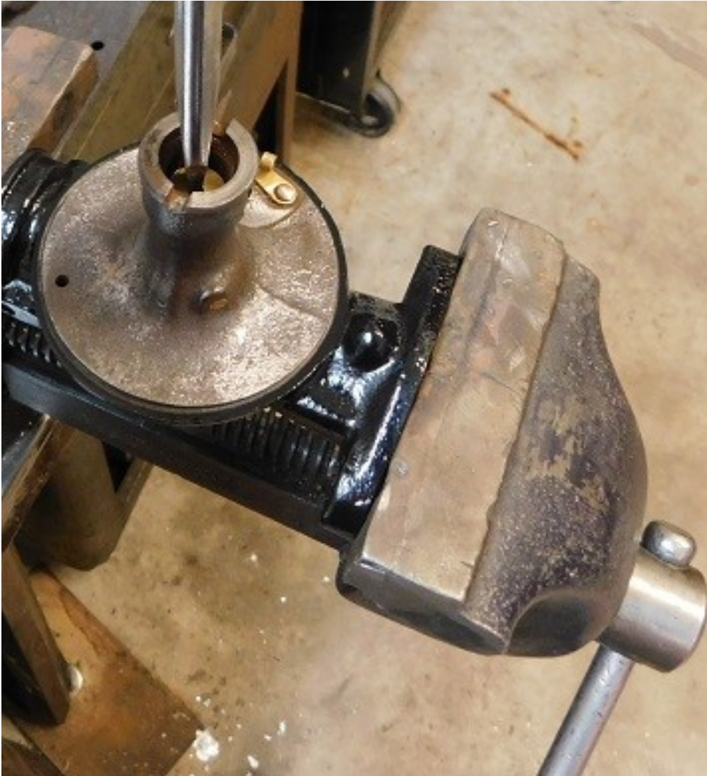
The new main jet is tightened with a normal screwdriver. The slot in the reproduction jet is smaller than the special screwdriver that fits the originals.
