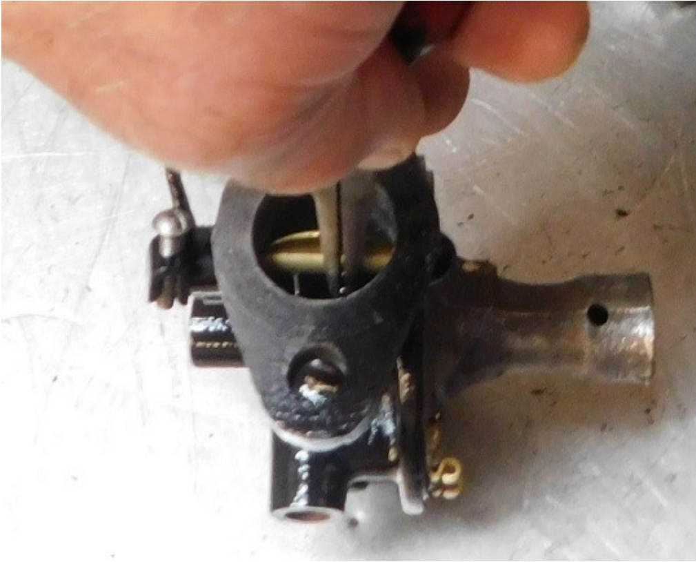
The throttle shaft and blade are installed. We made new clips from aircraft grade .041" stainless steel wire. Needle nose pliers are used to fold the ends inwards.
