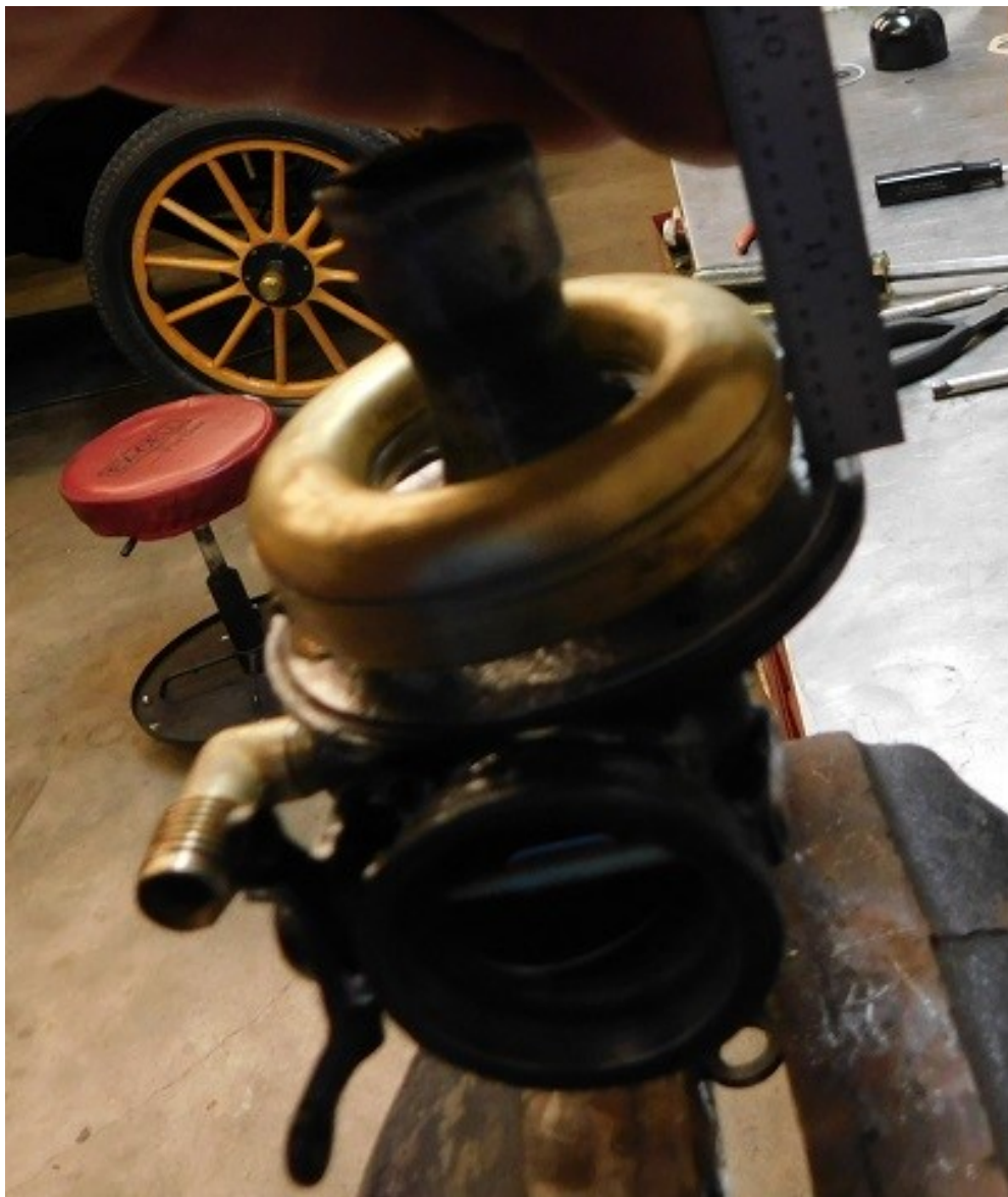
The float measures properly now at 1/4", and it is parallel with the bowl gasket surface all the way around too.
