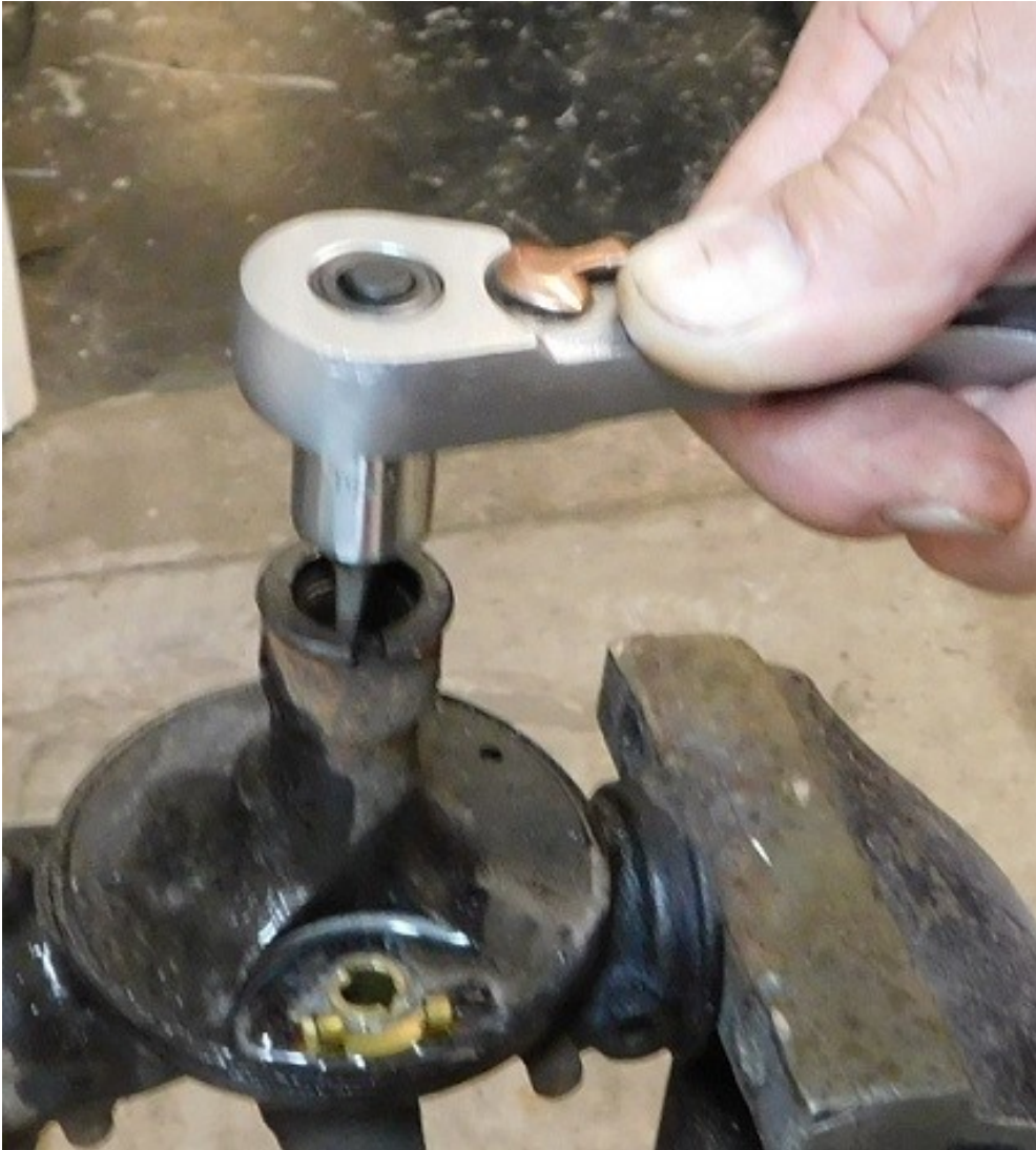
The main jet is removed using a specially ground flat blade screwdriver tip and a 3/8" ratchet after applying some penetrating oil.
