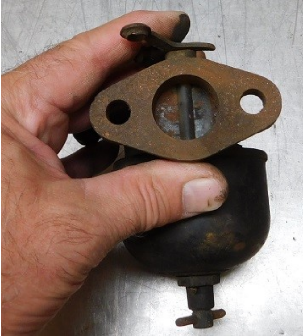
The throttle blade is the later style which does not use a clip; instead they have a bendable tab. To remove it the single inside tab is pushed to be inline with the slot.
