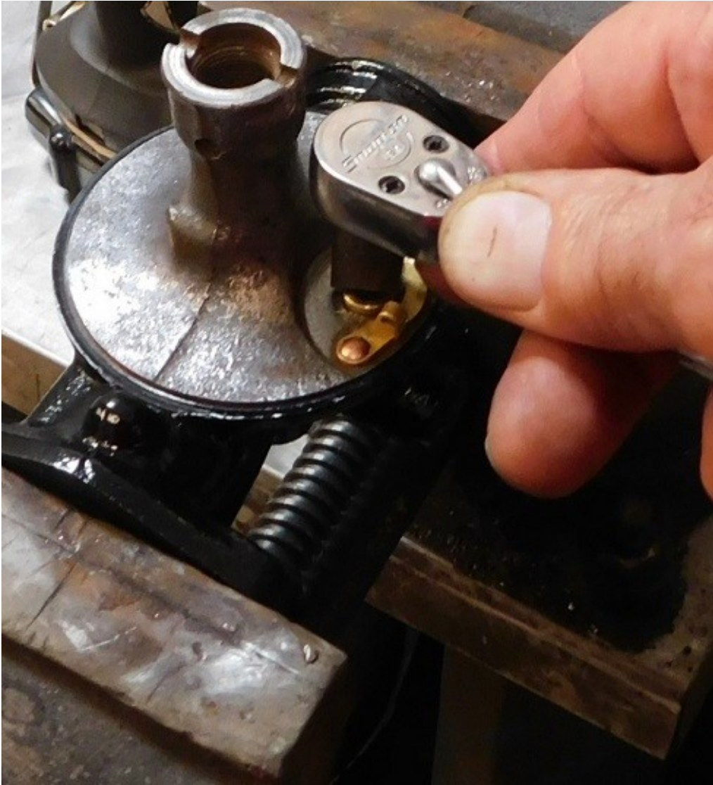
The fuel seat is tightened.
