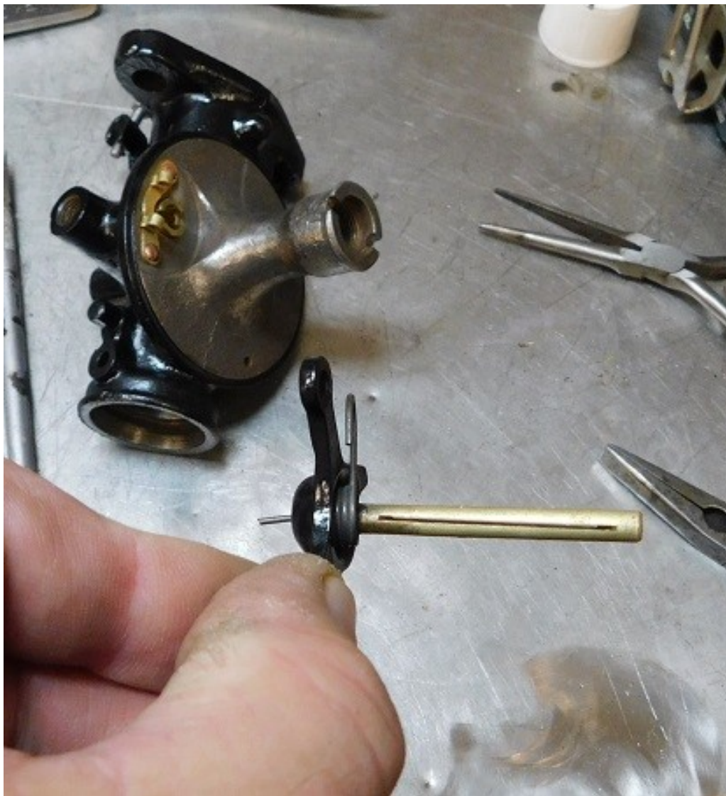
The new choke return spring is installed before the shaft is inserted. Then the blade and clip are installed just as the throttle blade was.
