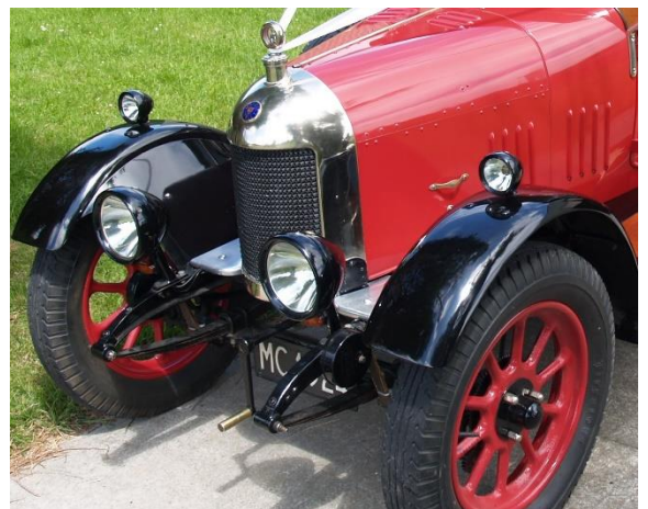
The indicator lights neatly installed under the headlight buckets.
